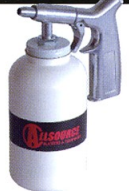
4001244 Bottle Blaster • Use abrasives or liquids • One quart capacity • 15 CFM @ 80 psi • 1/4" steel nozzle • Light weight & portable
