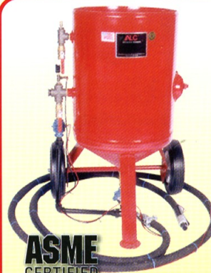
40011 Remote Blaster (F-600R) • Automatic tank closure • Adjustable abrasive flow valve • 80 - 125 psi Air Pressure • Pressure relief valve - 125 psi • Pressure gauge • Pressure relieving ball valve • Pressure choke valve • Manual pressure release • Dual remote media valves • Overall Height: 52" with 16" Wheels • Minimum Air Volume: 40 CFM @ 80 psi • 425 lbs. (skidded)
