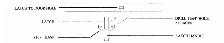
Assemble hasp to outside of front panel of cabinet. Close top door tightly against cabinet. Place latch to door hole. Hold latch handle straight out (90° from cabinet front). Mark holes for placement. Drill 11/64" holes in two places. Secure with two 8-32 screws from outside. Secure with two 8-32 hex nuts from inside.
