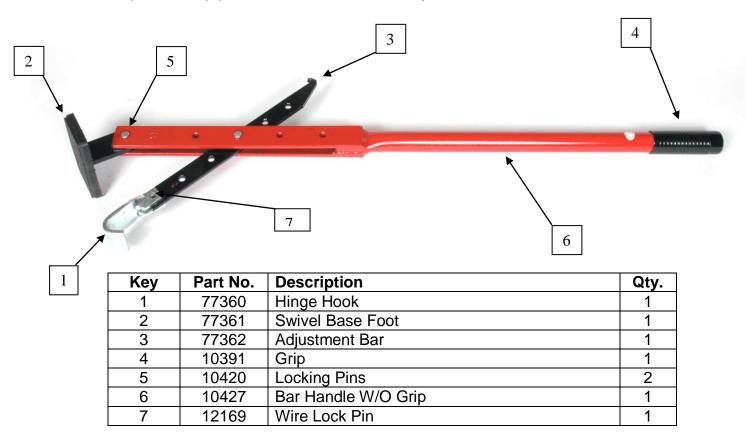
Slide pin through adjustment bar at desired hole location on tube assembly. Place swivel rubber base foot against a solid leverage point. Attach either the swivel hook or the adjustable bar end hook to damaged area and make pull. Apply even pressure. **Do not jerk or hammer on tube assembly.**
