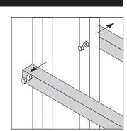
Horizontal posts are to be attached to the **outsides** of the vertical posts.
