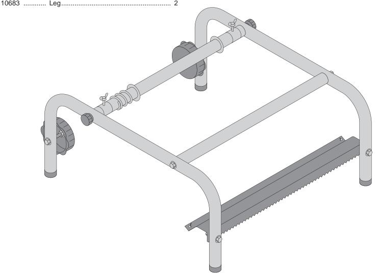
**STEP 1. Assemble the main frame tubing** using <sup>1</sup>/<sub>4</sub>"-20 X 2" bolts and <sup>1</sup>/<sub>4</sub>" washers. **Note the locations of all punched holes** in all tubing to ensure proper assembly. Assemble and install the Tape Spools. Follow the diagram below closely to ensure proper assembly of the Tape Spools. The order of the hardware is identical for both sides.
