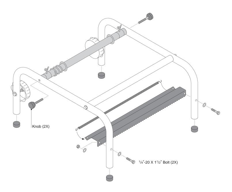
**Paper roll and tape spool placement**. Two Tape Spools are included so that you may conveniently run your tape along either end of your paper roll by simply adjusting the location of the paper roll along the Paper Bar.
