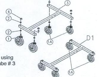
Install castors # 1 and locking castors # 1A using flat washers # 2 and lock nuts # 4 to base tube # 3 as shown in drawing D 1.
